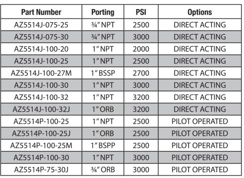
Direct acting - Rapid response, contamination tolerant & low leakage. Nominal flow range from 0 - 46 GPM
