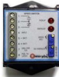
Available as 12 or 24 VDC, this switch is used to read the Engine RPM from the R terminal of the alternator. An adjustable potentiometer allows to set the engine RPM at which the unloading solenoids are cut off; thus, unloading the pump.
