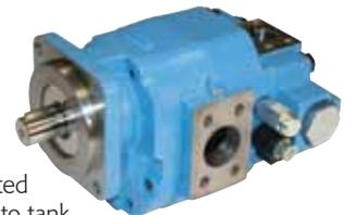
**The Versa-Pak Unloading System** limits the flow to the system while in use to prevent hydraulic overspeeding. While in the off mode the flow is diverted back to the tank at low pressures to control horsepower losses. Available with optional speed sensor and digital speed controller to further protect the hydraulic system.
