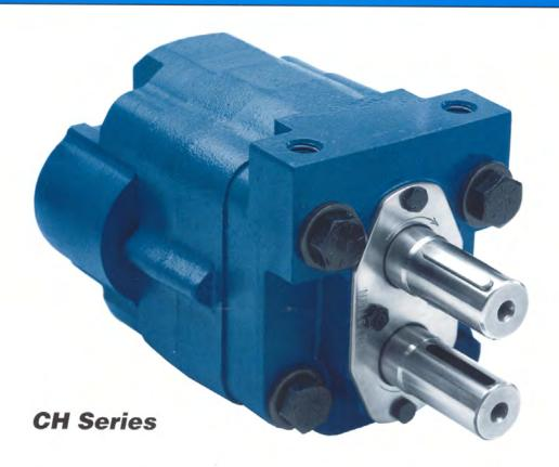
Permco's CH Series Gear Pumps have been designed specifically for the refuse truck market needs and are physically interchangeable with other manufacturers of this style pump. The CH Series Pumps are made of high strength cast iron and alloy steel incorporating Permco's rugged and dependable gear pump design. CH Pumps are pad-mounted with double 11/8 inch drive shafts and large port end covers with 11/2 inch NPT inlets and a choice of 3/4 inch or 1 inch O-ring outlets.
