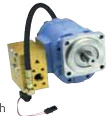
**The Versa-Pak Dry Valve System** incorporates an air operated dry valve which permits hydraulic operation while the vehicle is in motion. It reduces fuel consumption during the off mode and eliminates heat build-up associated with "live" systems in the on mode. Available with optional speed sensor and digital speed controller to further protect the hydraulic system.
