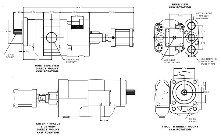
The third line sleeve is installed in the pump, therefore, the return port must be plumbed back to tank, below the oil line at all times.
